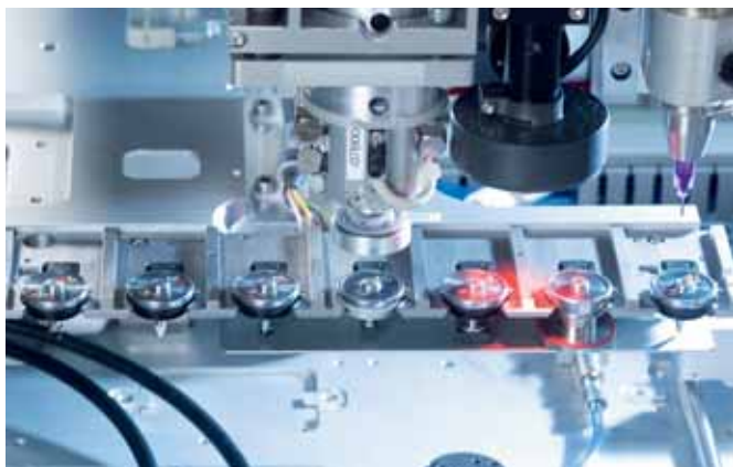
Automatic 7-slot tool changer (expandable to 14 slots)
