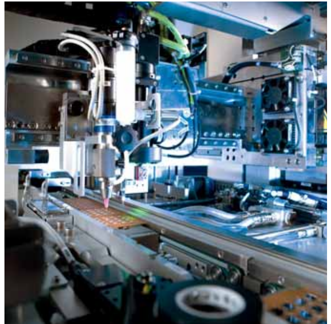
View on the integrated dispense axis and dispenser unit for parallel dispensing and pick&place in combination with the main axis (not shown here).
